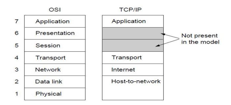
Fig. 1-21. The TCP/IP reference model.
