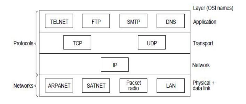
Fig. 1-22. Protocols and networks in the TCP/IP model initially.
